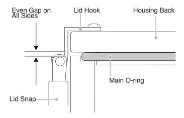
**6.** Check the o-ring seal. The o-ring should form a uniform, solid line around the back of the housing. There will be a small, even gap around the housing between the housing back and the housing front.
