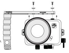
4. With your free hand, insert and rotate the 1/4-20 x 1/2" screws clockwise until threaded into the housing mounts. Finish tightening the tray to the housing using a flathead screwdriver. Do not overtighten.
